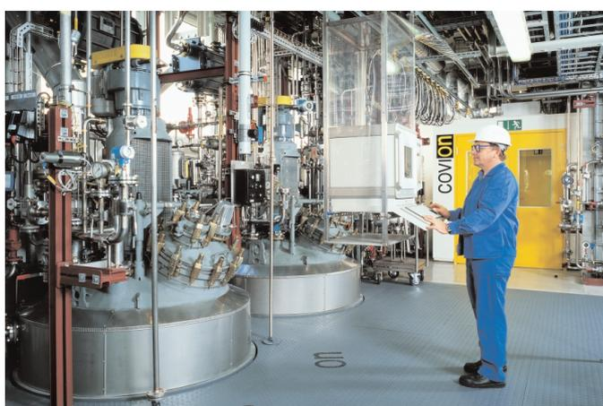
*Illustrations of the up-scaling from development to production equipment for OLED materials*
