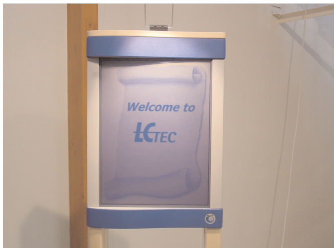
An example of a CTLC signage display made in LC-Tec
