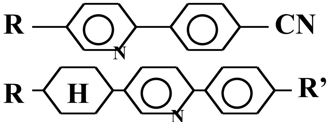
Fig.10. Chemical structure of bi- and tricyclic mesogenic pyridine derivatives
