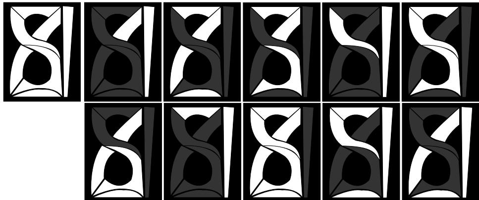
Fig.2. Indicators for characters displaying which provide detection and correction of single mistakes.
