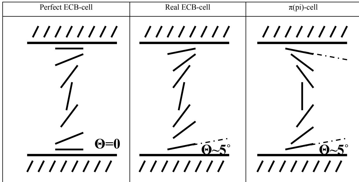
Fig.11. LC director structure inside different ECB-cells.
