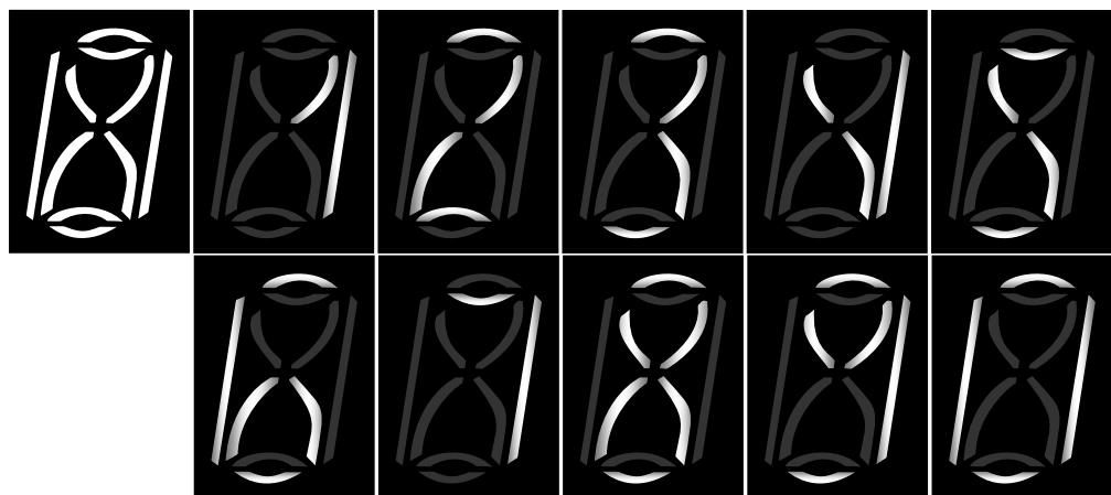
Fig.3. A character display with minimized number of switching segments.
