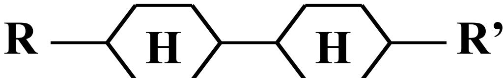
Fig.8. Chemical structure of bicyclohexanes (BCH)
