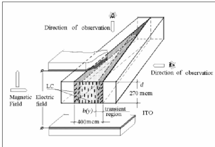
FIGURE: General scheme of the LC cell.
