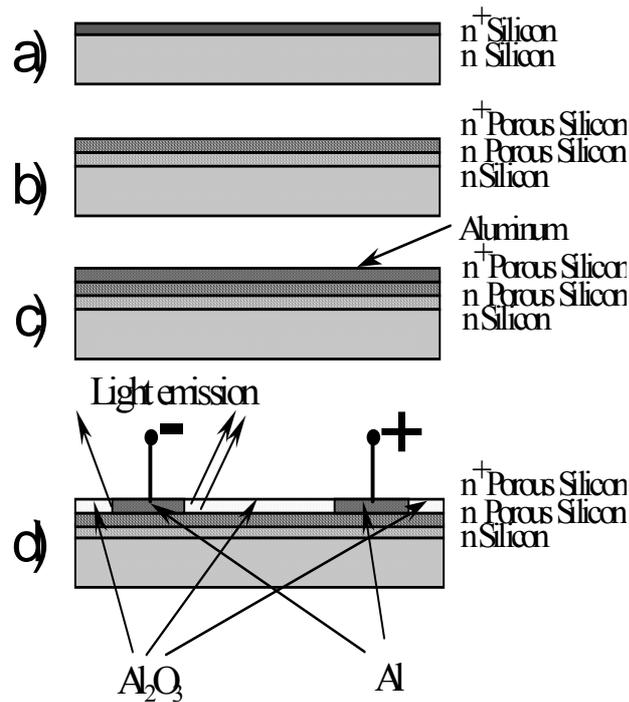
Schematic view of fabrication process and a PS LED structure: a) n-type silicon wafer with n<sup>+</sup>-diffused layer; b) after anodization in transition regime, PS is formed both in n<sup>+</sup>- film and in a substrate layer; c) aluminum layer is deposited by magnetron sputtering; d) the final structure after photolithography and sub-sequent aluminum anodization. Light emission at the edge of negative biased pad is evidenced.
