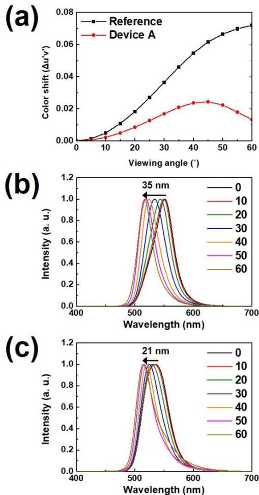
**Figure 5.** (a) Angular color shift ( $\Delta u'v'$  in CIE 1976 color system); (b) angular EL spectrum shift of reference; (c) angular EL spectrum shift of Device A.
