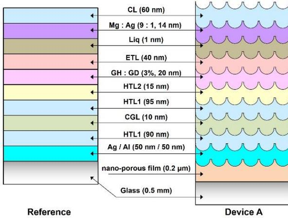
**Figure 3.** Schematic device structure comparison.
