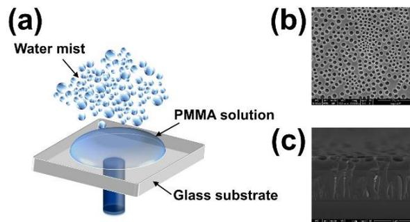
Figure 2. Schematic diagram of preparation of nano-porous film; (b) SEM image of the front view of nano-porous film; (c) SEM image of the cross section of nano-porous film.
