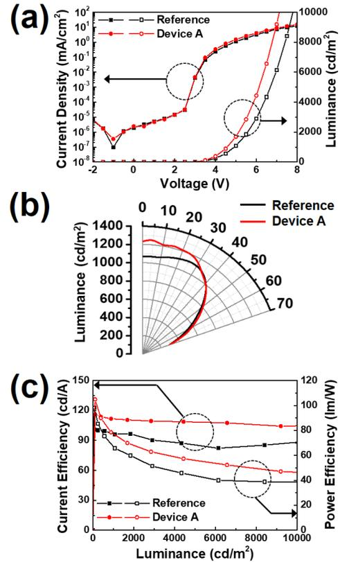
**Figure 4.** (a) J-V-L characteristics of devices; (b) angular luminance distribution characteristics of devices; (c) luminance-current efficiency and power efficiency characteristics of devices.
