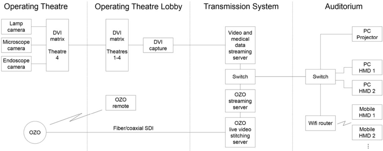
**Figure 2.** Block diagram of the image delivery setup for the augmented VR demonstration.
