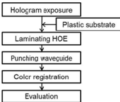
Figure 2. Process flow diagram of the plastic holographic waveguide
