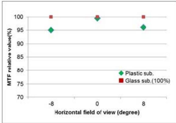
**Figure 8.** MTF result comparison of the plastic substrate to the glass substrate
