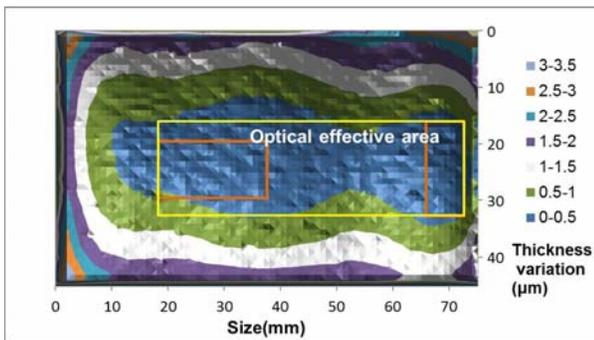
Figure 3. Thickness variation result of the plastic substrate (The color coding denotes 0.5µm contours)
