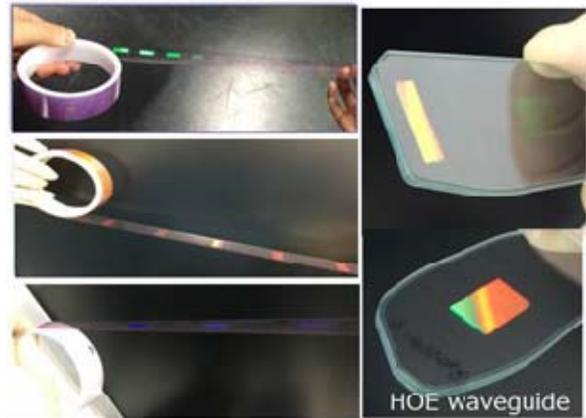
Figure 4. Green, Red & Blue HOE in the roll-film, and Full-color plastic holographic waveguide
