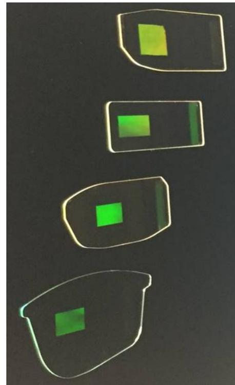
Figure 5. Shape variations of the plastic holographic waveguide in a punching process
