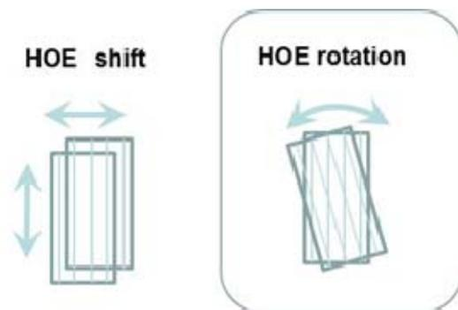
Figure 6. Variations of the HOE shift in a laminating process
