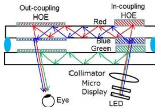
**Figure 1.**An optical structure of the holographic waveguide combiner
