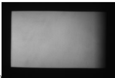
Fig. 2. Example image of vignetted full-screen pattern (a), and (b) the boundary area determined by edge detection.
