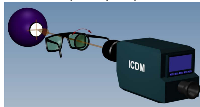
Fig. 3. Testing glasses polarization quality using a uniform source and a good linear polarizing filter.
