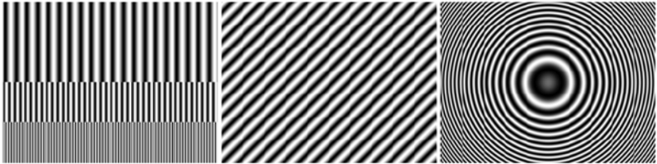
Fig. 6. Resolution patterns at a given depth \mathcal{X} with sinusoidally varying gray levels. Note all grey levels have the same depth
