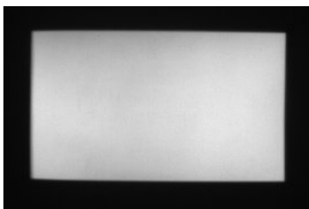
Fig. 1. Example image of unvignetted full-screen pattern near the nominal eye-point (a), and (b) the boundary area determined by edge detection.
