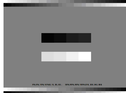
Fig. 1. Pattern (SET01S50) to set up the front-projector.
