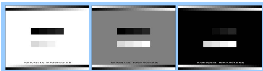
FIGURE 4.5. Patterns for adjustment of the near-white and near-black gray levels.
