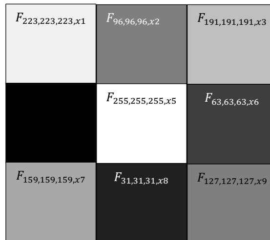
Fig. 4. Example of a test image with sub-patches, each with different combinations of mid-gray values and depths.
