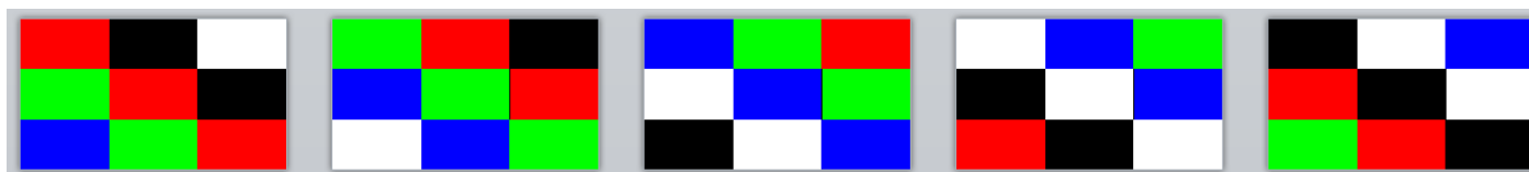
FIGURE 2.2. Test patterns for color-tile characterization.
