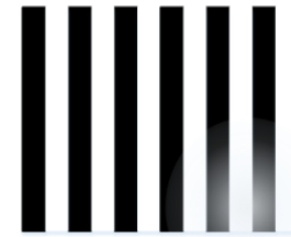
Fig. 5. Grille pattern showing effect of veiling glare.
