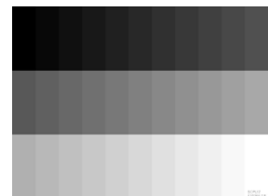
FIGURE 3.5. Pattern with black at corner but with content elsewhere (50 % average pixel level). SCPL17_####x####.png
