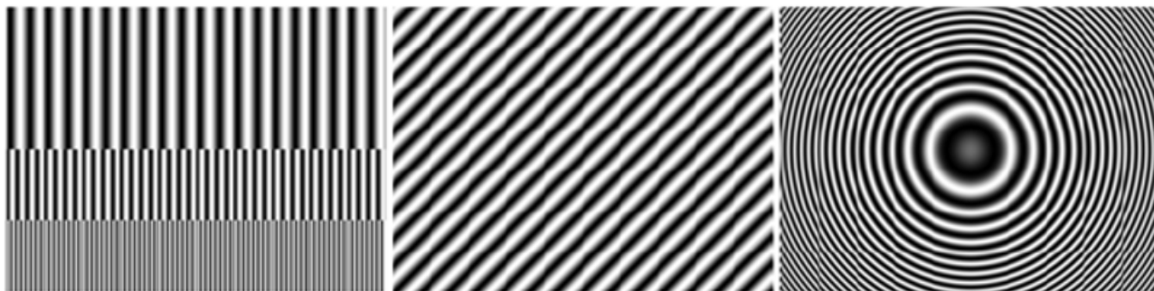
Fig. 6. Resolution patterns at a given depth x with sinusoidally varying gray levels. Note all grey levels have the same depth
