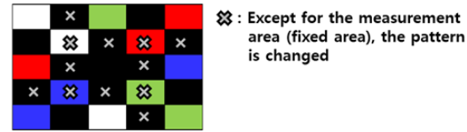
FIGURE 10.19. Initial measuring points in test pattern
