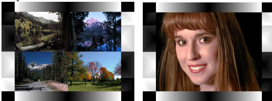
FIGURE 3.4. Static images of scenes and especially faces are ways to check if the gray scale is rendered properly. You may see a problem in a face image that is not discernible in a gray-scale ramp or color-scale ramp or even a natural scene. These and other images, including faces, are available for download at DOI 10.55410/LGAM8989 .
