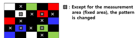
FIGURE 10.25. Initial measuring points in test pattern
