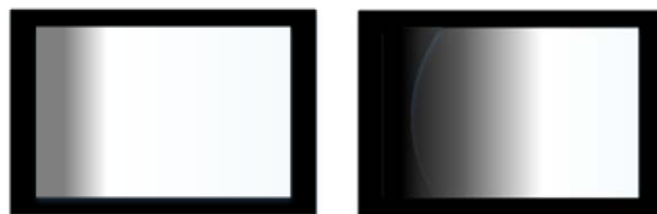
Fig. 3. a) Full-field Luminance as LMD approaches the edge of the eyebox; b) Luminance reduced to ~50% at center of field. Note: edge of exit pupil may be visible.
