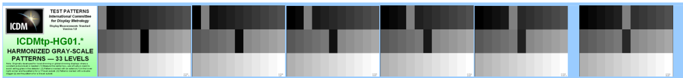
Fig. 6. Beginning sequence of snaking constant-pixel-level patterns in ICDMtp-HG01.* containing 33 gray levels.
