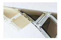
**Plastic backplane**. The backplane applies the charge pattern to the e-paper layer. Standard displays use a glass backplane, which can crack very easily. Instead, popSLATE uses a plastic backplane. This technology makes our displays shatter-proof, lightweight, and delightfully curvable.
